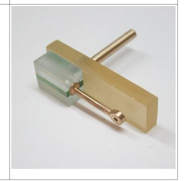
Cutting the crankshaft wheel
